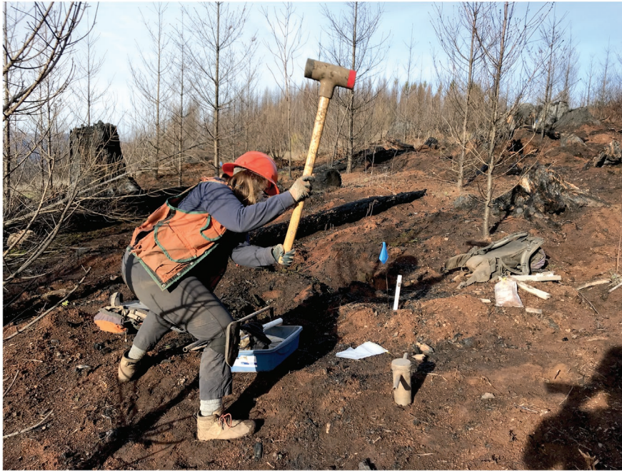
Hammering the soil core into the soil to collect a sample down to 30 cm. Photo courtesy of K. McCool.
