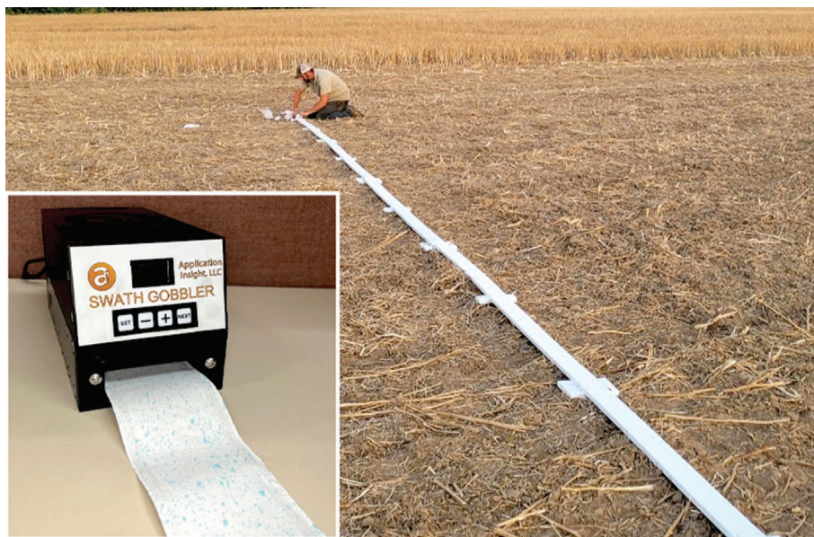
Setting up the equipment for Mark Ledebuhr's fast and inexpensive swath uniformity and coverage evaluation method. Inset: The Swath Gobbler analyzes continuous rolls of paper from the swath evaluation method and calculates percent coverage and hits per area. The blue dots on the paper show a typical drone spray pattern. Photos courtesy of Mark Ledebuhr, Application Insight, LLC.
