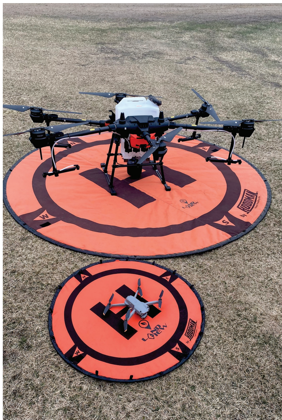
Drones come in all sizes. The small drone is the DJI Air 2S, which is used for observing crops. The large drone is the DJI Agras T20 spray and spread. Photo courtesy of Markus Weber, LandView Drones.
